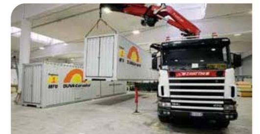
A complete foaming line, able to produce CORAFOAM® PIR foam blocks within the space of 4 containers, that can be shipped and transported on customer's site to produce large quantities of foam, while saving transport costs of bulky products. The most customer-oriented solution by DUNA Group to support the largest cryogenic projects in faraway locations. DUNA technical Team takes care of the Unit installation and operation, assuring constant supervision and strict quality control.
